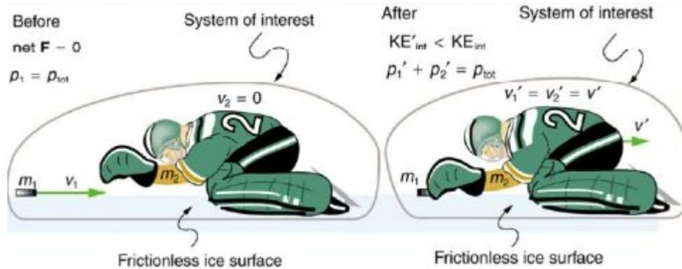
Find the recoil velocity of a 70.0 kg ice hockey goalie, originally at rest, who catches a 0.150 kg hockey puck slapped at him at a velocity of 35.0 m/s
