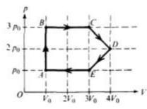
An ideal gas undergoes a cyclic process as shown on the graph above of pressure p versus volume V.
