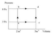
59. In the Pressure versus Volume graph shown, in the process of going from a to b 60 J of heat are added, and in the process of going from b to d 20 J of heat are added. In the process of going a to c to d, what is the total heat added?
