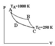
50. A monatomic ideal gas is used as the working substance for the Carnot cycle shown in the figure. Processes A  $\rightarrow$  B and C  $\rightarrow$  D are isothermal, while processes B  $\rightarrow$  C and D  $\rightarrow$  A are adiabatic. During process A  $\rightarrow$  B, there are 400 J of work done by the gas on the surroundings. How much heat is expelled by the gas during process  $C \rightarrow D$ ?
