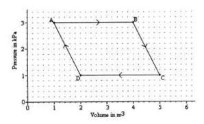
71. A sample of gas is caused to go through the cycle shown in the pV diagram shown above. What is the net work done by the gas during the cycle?
