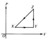
A thermodynamic system is taken from an initial state X along the path XYZX as shown in the PV-diagram.
