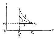
A certain quantity of an ideal gas initially at temperature  $T_0$ , pressure  $p_0$ , and volume  $V_0$  is compressed to one-half its initial volume. As shown above, the process may be adiabatic (process 1), isothermal (process 2), or isobaric (process 3).
