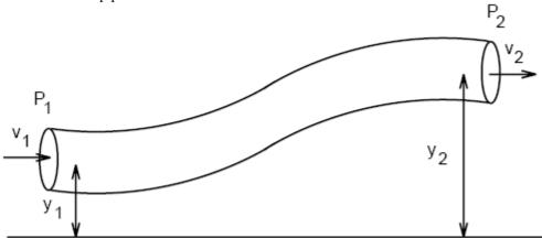
The pipe changes height from  $y_1 = 2$  meters to  $y_2 = 3$  meters. Since the areas are the same, we can say  $v_1 = v_2$ . Which of the following is true?
